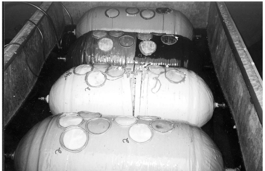
III. 4 – Stress corrosion cracking – testing of glass fibre wrap on pressurized tanks.
