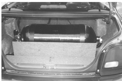
Ill. 2 – Fully-wrapped CNG cylinder mounted on a vehicle.
