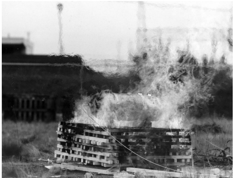
III. 3 – Bonfire test of steel cylinder to evaluate the performance of pressure relief devices.
