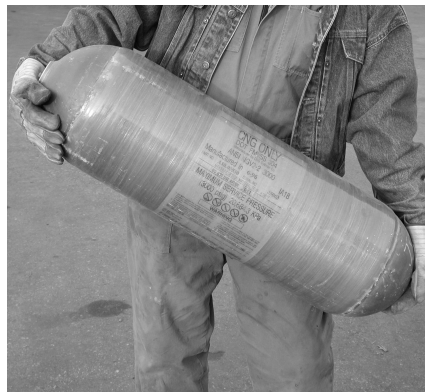
III. 1 – CNG cylinder – aluminium liner hoop-wrapped with glass fibre composite.
